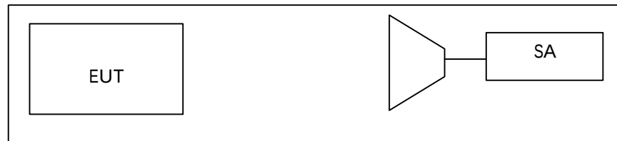
Figure A-3. Test Instrument & Measurement Setup
