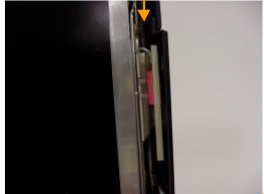
Auxiliary antenna Dual Band Meander antenna P/N: 08K4084
