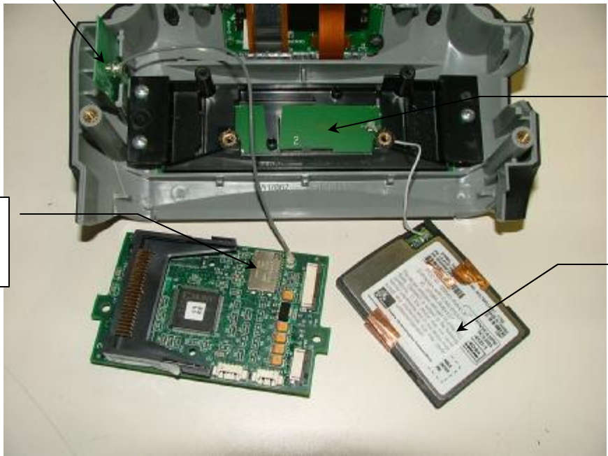
RF Carrier Board with RW4137 Removed
