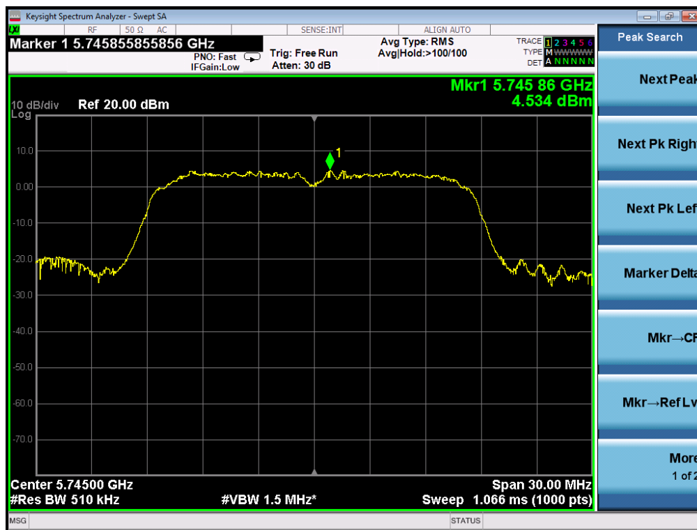
TEST PLOT OF SPECTRAL DENSITY FOR 5745MHz AT CHAIN 2
