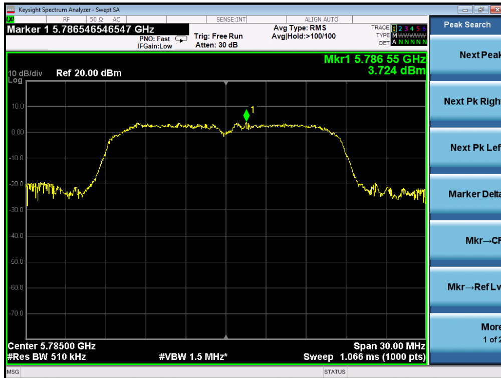
TEST PLOT OF SPECTRAL DENSITY FOR 5785MHz AT CHAIN 2
