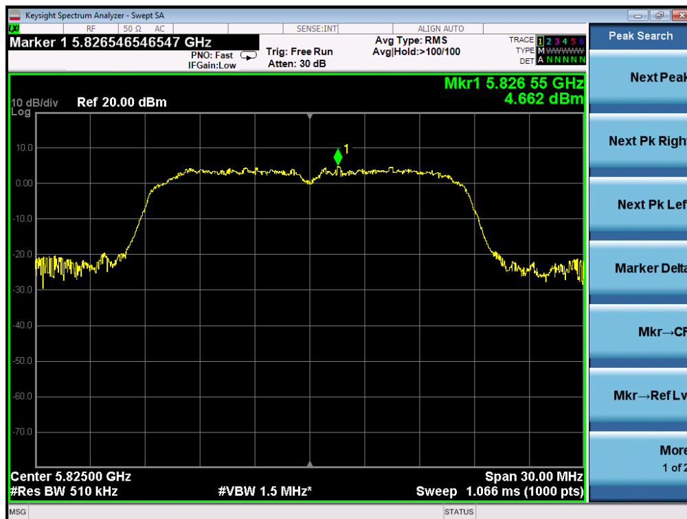
TEST PLOT OF SPECTRAL DENSITY FOR 5825MHz AT CHAIN 2
