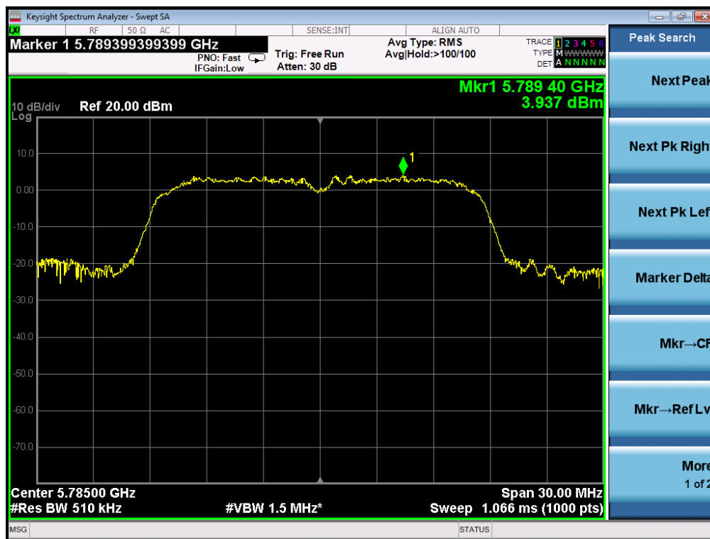
TEST PLOT OF SPECTRAL DENSITY FOR 5785MHz AT CHAIN 2
