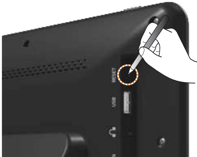
To reset the system, use a clip or a pin to press into the RESET button.
