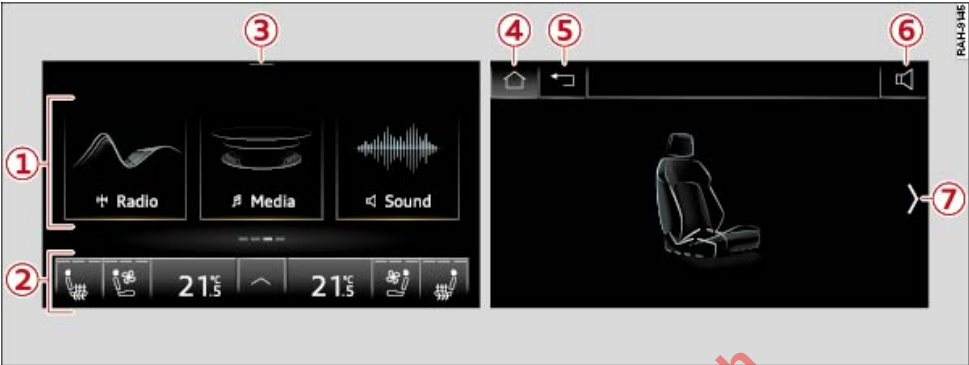
Fig. 22 Display: Example of home screen (left) and sub-menu (right)
