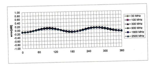
Axial Isotropy Error < ± 0.2 dB
