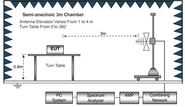
(C) Radiated Emission Test-Up Frequency Above 1GHz
