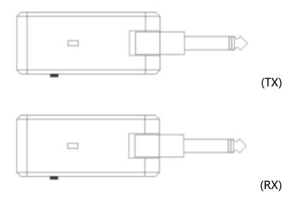
Press and hold the pairing button on both the transmitter and receiver for more than 2 seconds. If the blue lights on both the transmitter and receiver turn on, it indicates a successful pairing. The transmitter will select the best channel when turned on, and the receiver will automatically follow the transmitter.
