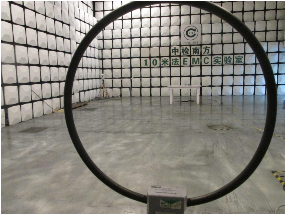
Radiated Emission Test setup photos
