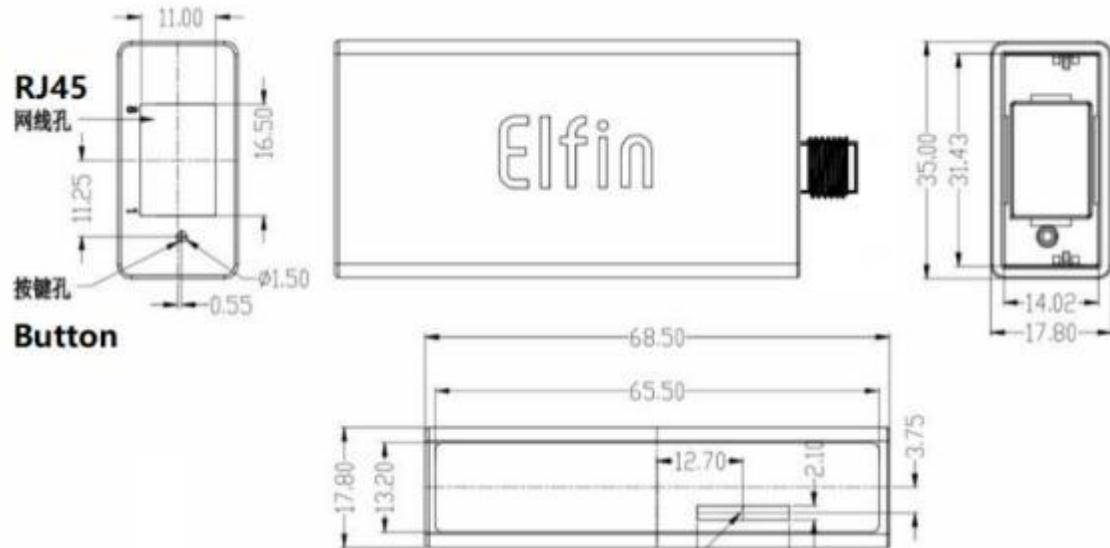
Figure 7. Elfin-EW4XB Mechanical Dimension
