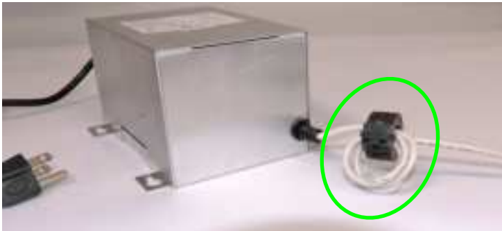
Figure 14: Optional Ferrite Core Placement, Near PSU Adapter
