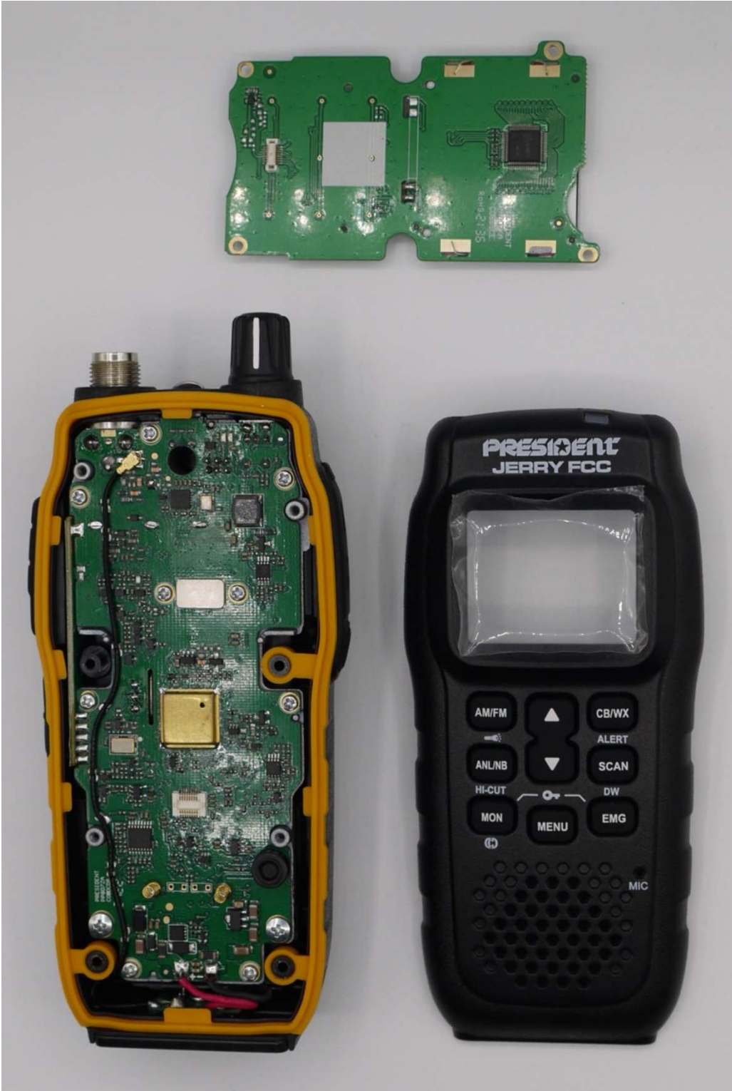
Figure E17.1 – Internal, Front Cover Removed
