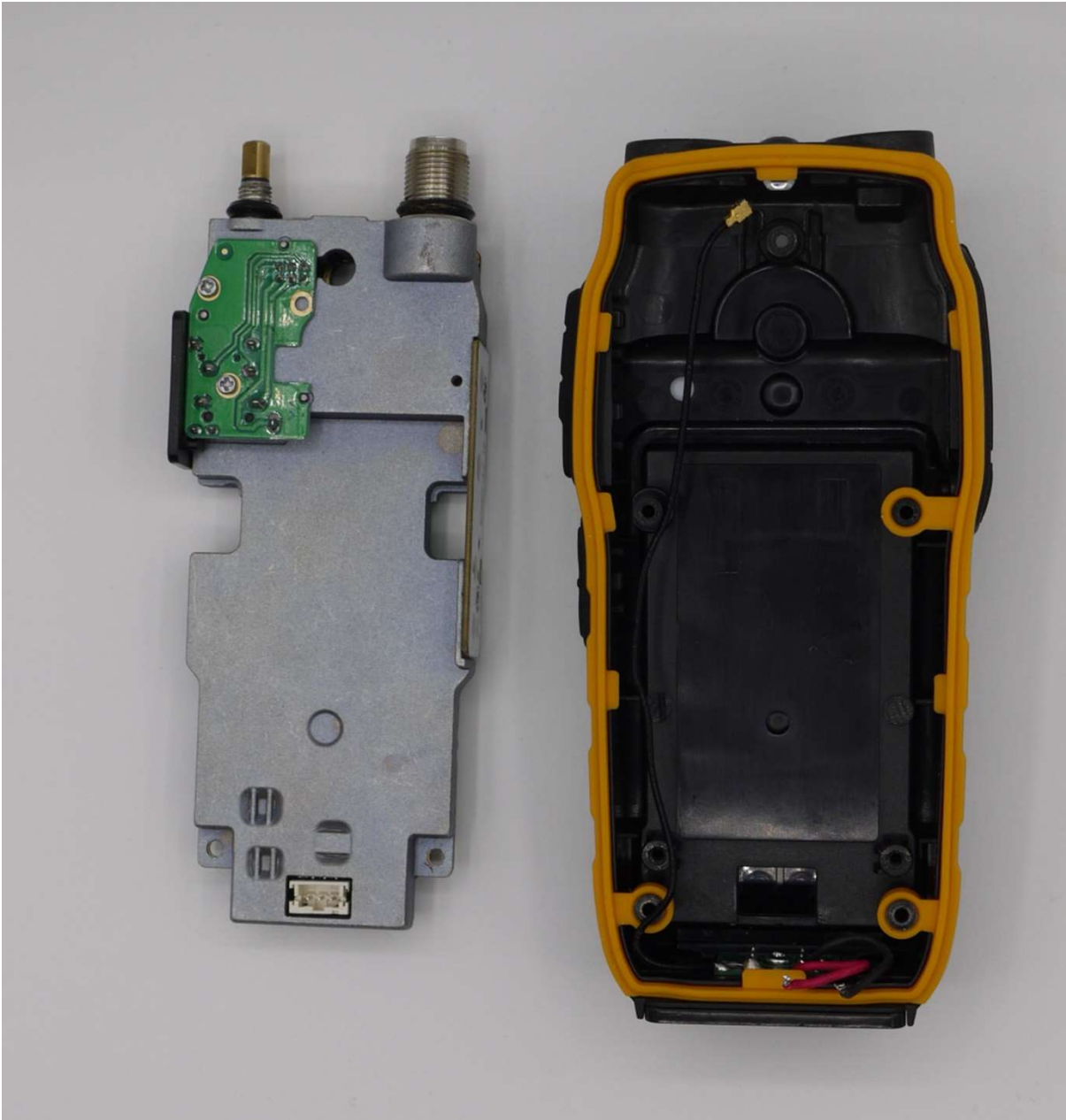
Figure E17.4 – Internal, Back Cover Removed
