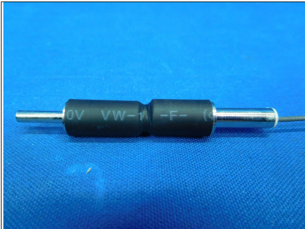
WLAN antenna No. 1
