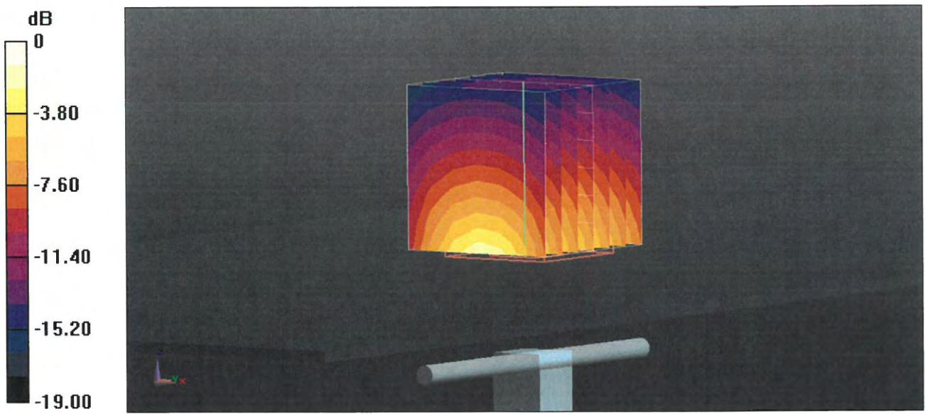
$$0 \text{ dB} = 14.9 \text{ W/kg} = 11.73 \text{ dBW/kg}$$
