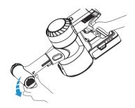
Activate the appliance on MAX mode, and rotate the side cover to clean the dirt pre-filter. Then remove the filter for backup after cleaning.
