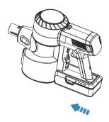
Slide the battery into the bottom of the main body. The battery will click into position when correctly fitted.
