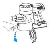
When finished, press the release button on the side of the dustbin and empty the contents.
