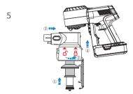
Insert the clean pre filter into mesh filter properly, a "click" sound will be heard once right into place. Install the clean dustbin and filters back into the main body, then reattach the dustbin cover.
