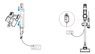
Connect the adaptor to docking station and outlet.
