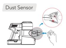
To avoid dust accumulation which can affect cleaning performance, wipe the suction mouth with a damp cloth.
