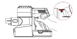
Press the switch button, the appliance will start to work.
