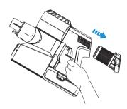
Press the HEPA release button and gently pull out the HEPA to remove the dust. Do not start the appliance when the HEPA is not installed.
