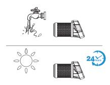
The HEPA can be washed under running water if necessary, and should be dried completely before reinstalling.
