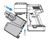
Incline the dustbin, the slot on the dustbin towards the hook on the main body. Push upward until the hook fixed into the slot. A "click" sound will be heard when it has been successfully accomplished.
