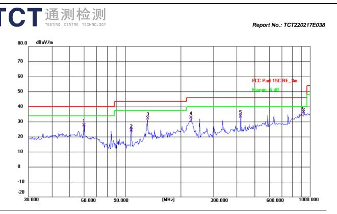
Site #1 3m Anechoic Chamber Limit: FCC Part 15C RE\_3m Polarization: Vertical Power: DC3.8V
