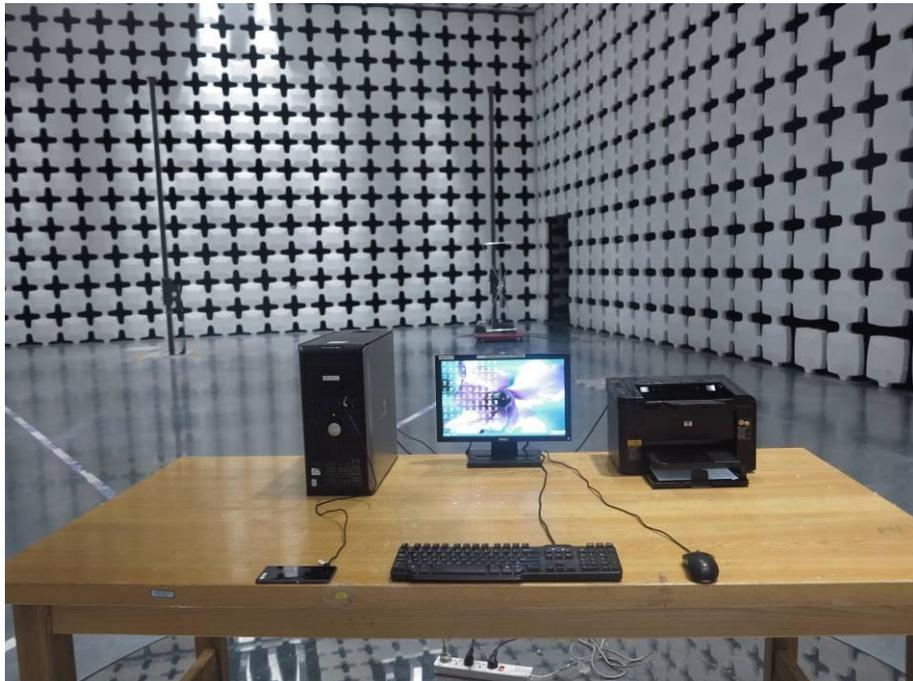
**Picture C-7: Radiated emission (PART15B)**
