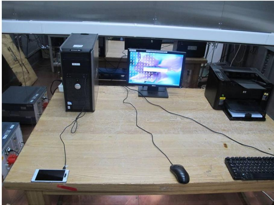
**Picture C-8: Conducted emission (PART15B)**
