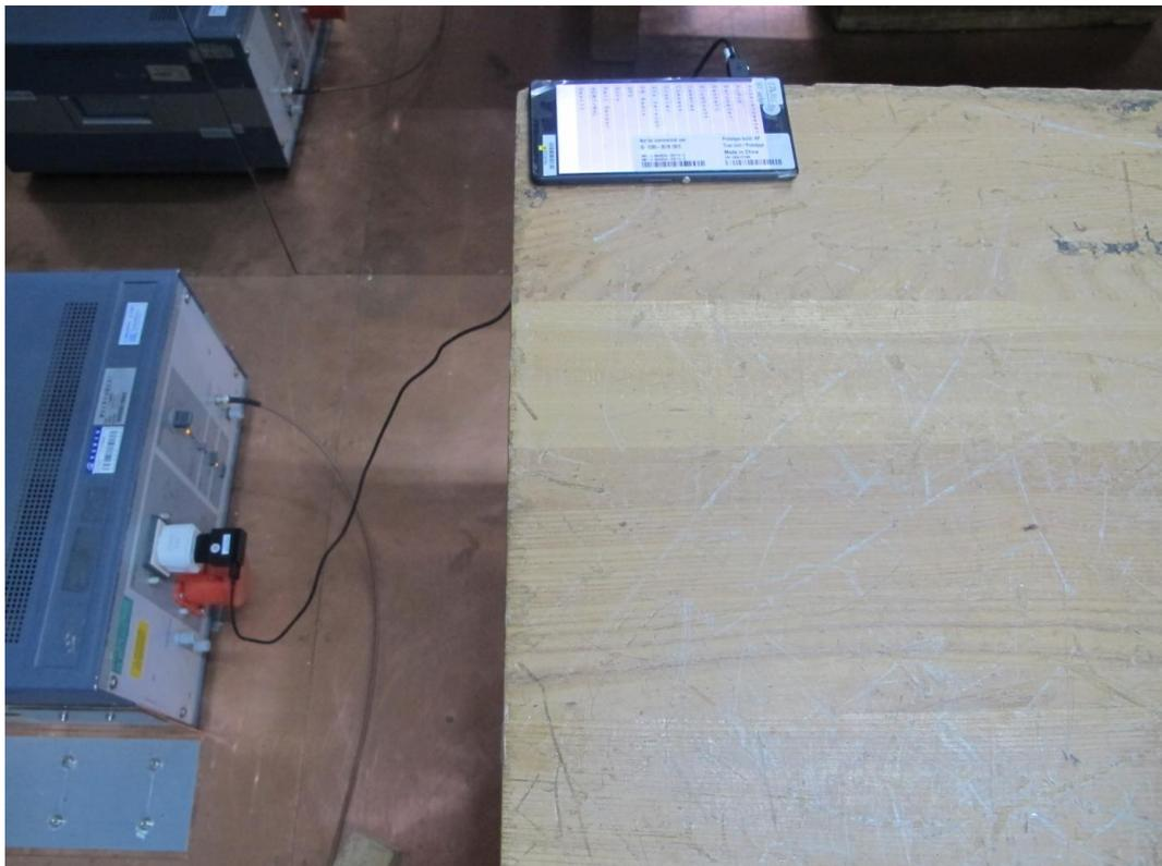
**Picture C-3: Conducted Emissions Measurements (PART15C)**
