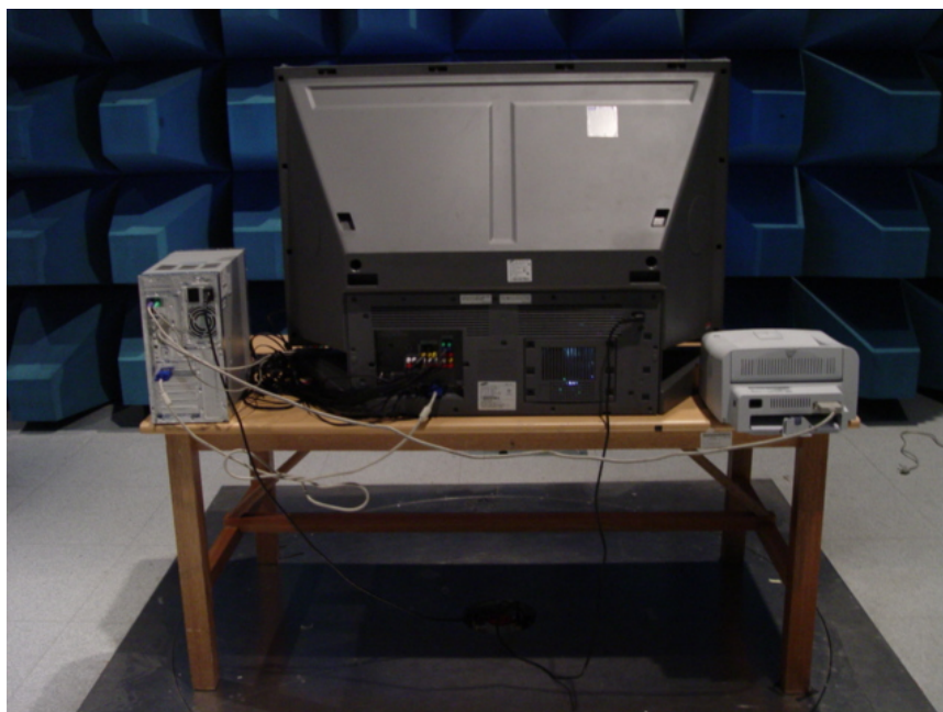
Picture 3. Radiated Emission (rear view)
