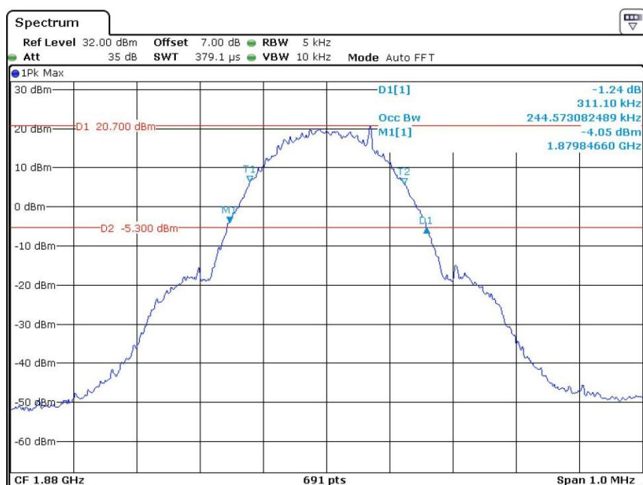
**26 dB Emissions & 99% Occupied Bandwidth for GSM (GMSK) Mode, High channel**
