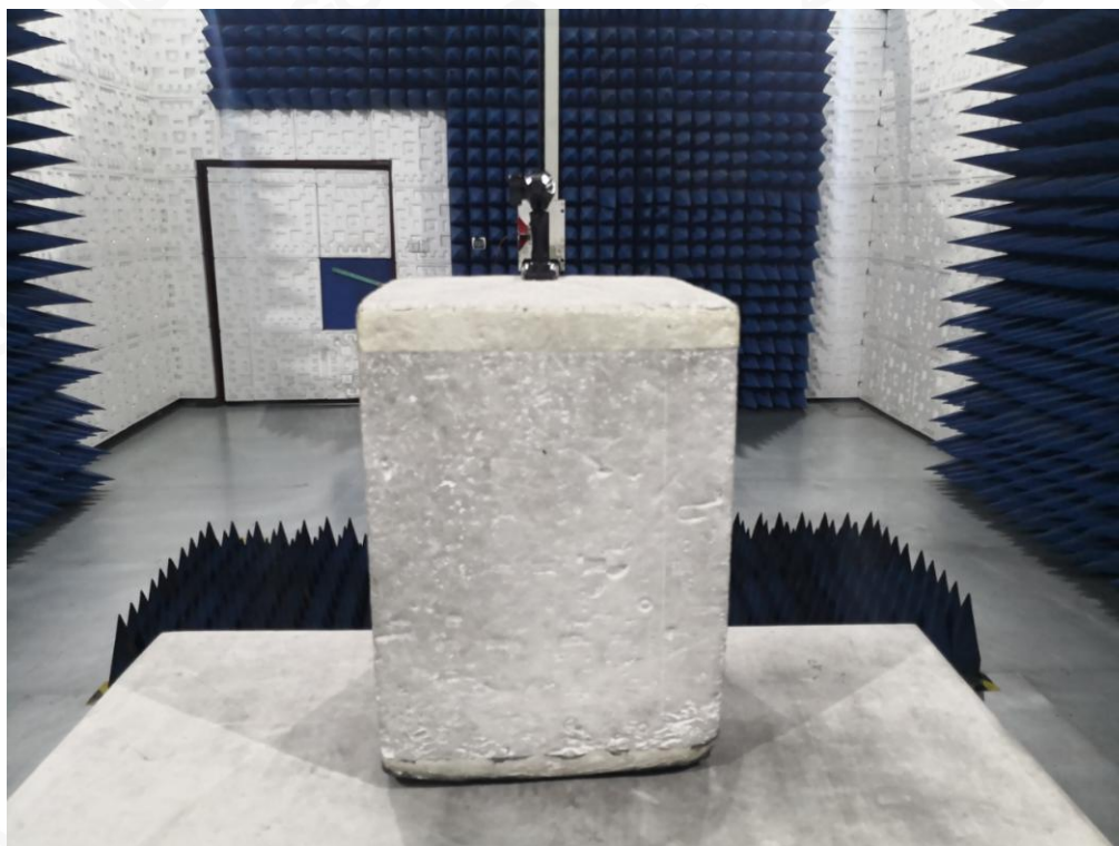
FCC RADIATED EMISSION TEST SETUP ABOVE 1GHZ
