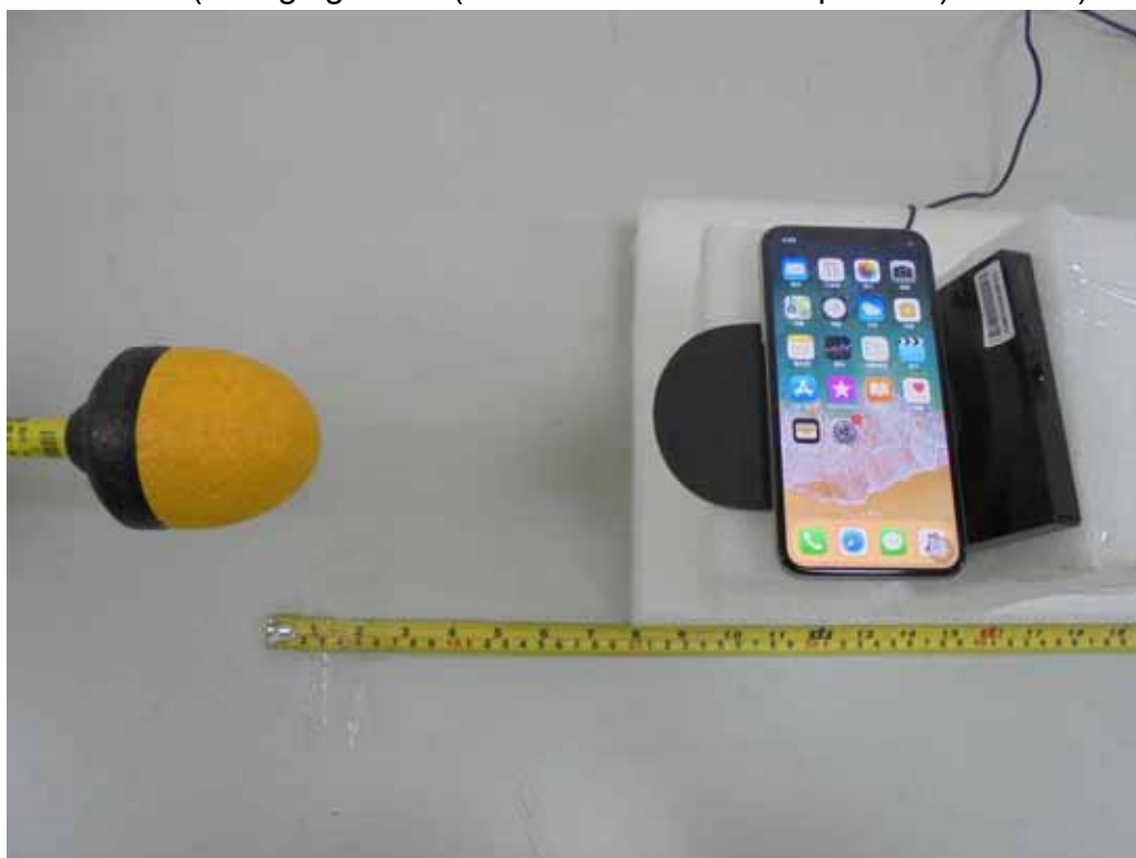
E-Field (Charging Mode (iPhone in the lie-down position) - Z-axis)
