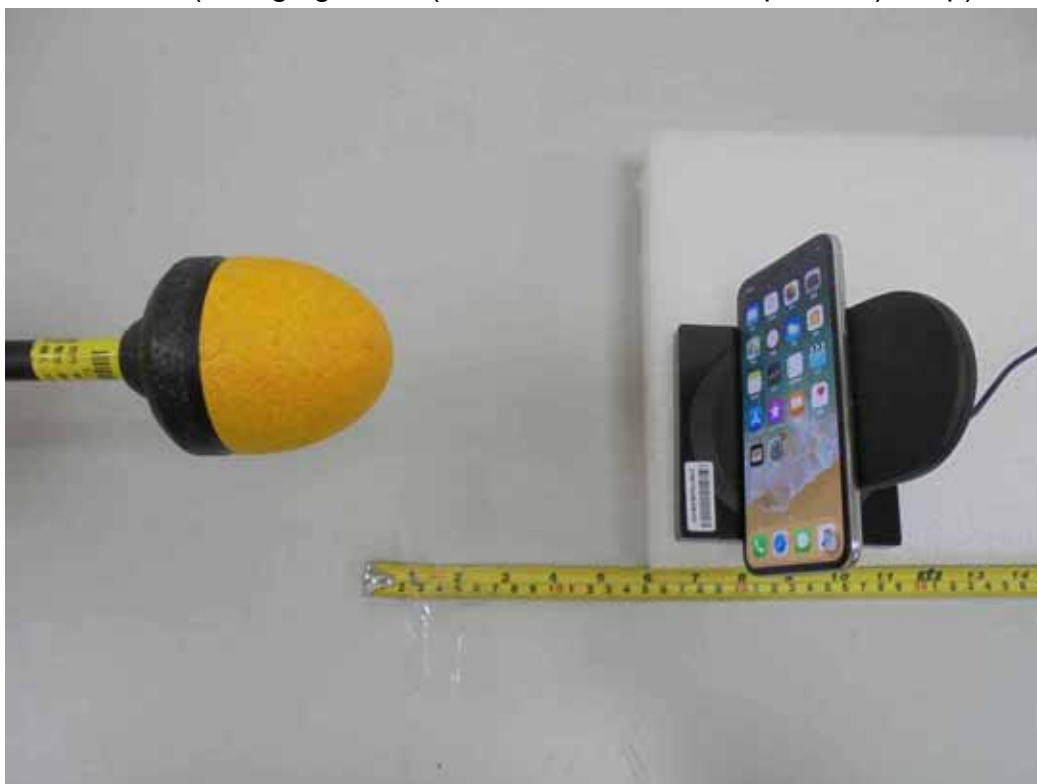
E-Field (Charging Mode (iPhone in the lie-down position) - Top)
