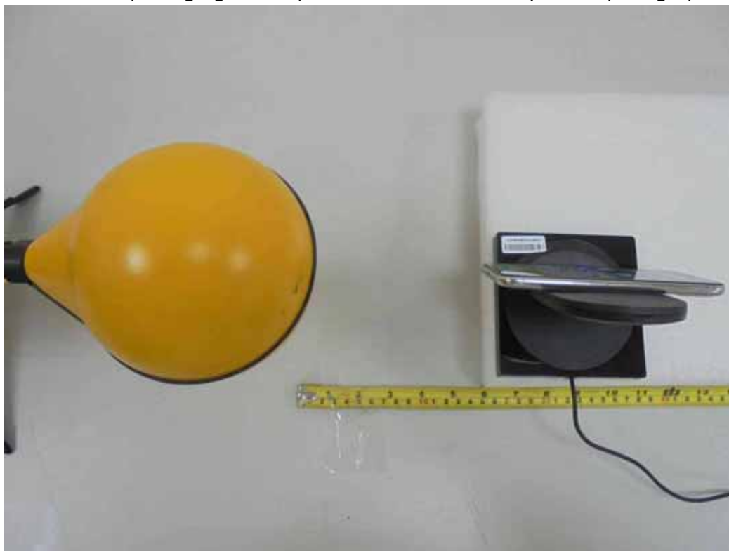
H-Field (Charging Mode (iPhone in the lie-down position) - Right)
