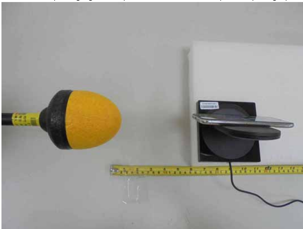
E-Field (Charging Mode (iPhone in the lie-down position) - Right)
