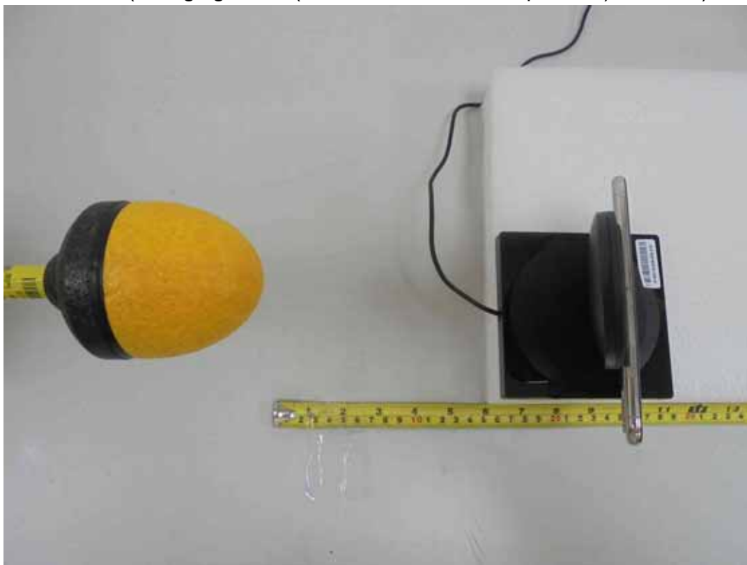
E-Field (Charging Mode (iPhone in the lie-down position) - Bottom)
