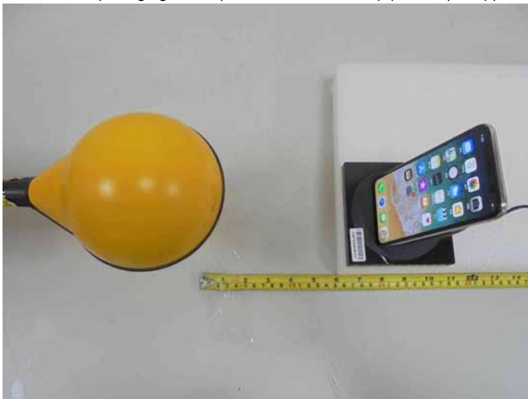
H-Field (Charging Mode (iPhone in the stand-up position) - Top)
