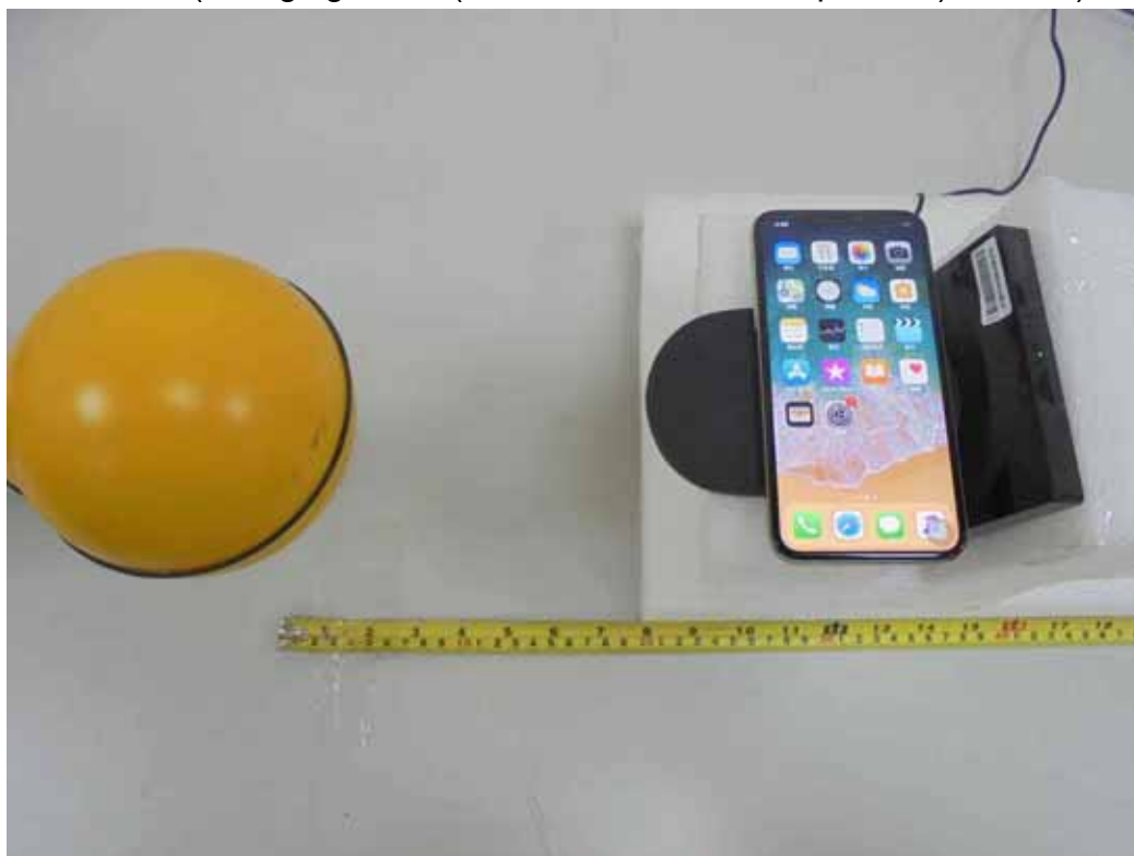
H-Field (Charging Mode (iPhone in the lie-down position) - Z-axis)
