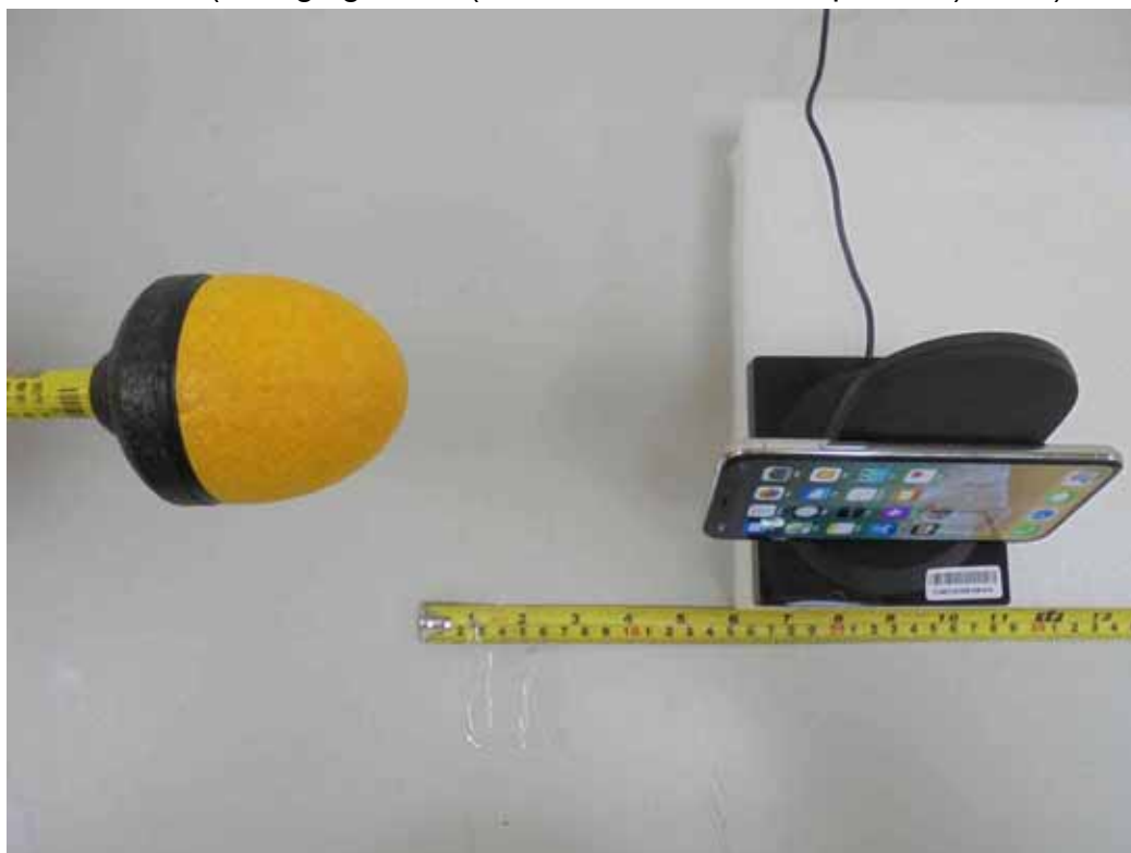
E-Field (Charging Mode (iPhone in the lie-down position) - Left)
