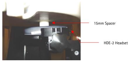
Note: the 15mm spacer was removed before the SAR measurement.
