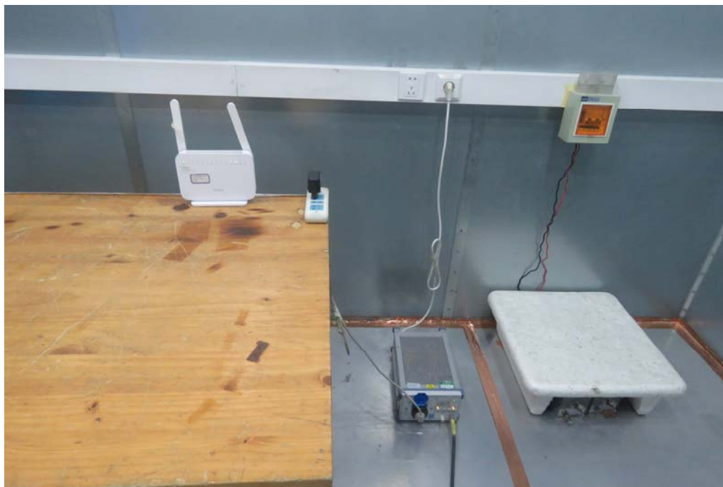
Picture 2 Conducted Emission Test Setup
