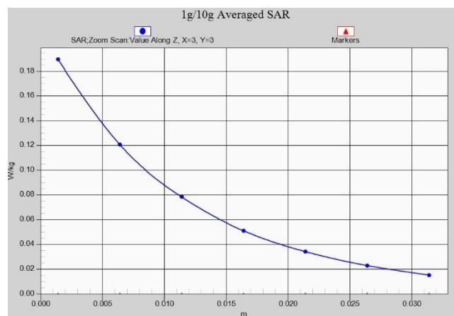
Z-Scan at power reference point (WCDMA1900)
