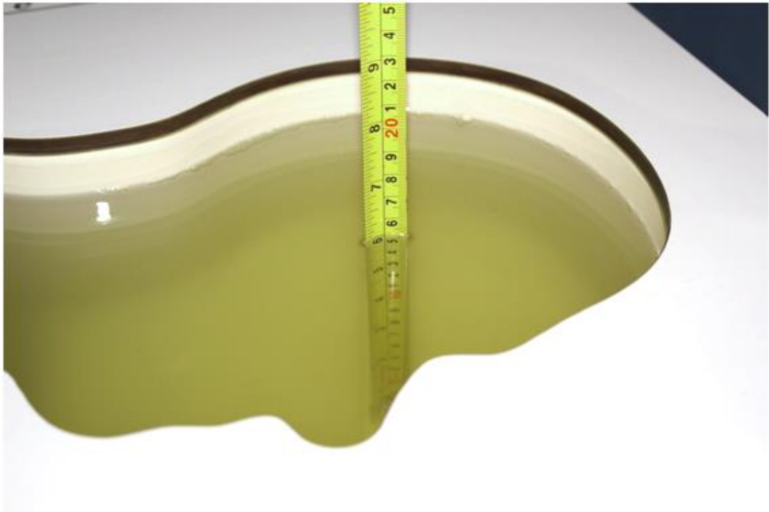
Picture 7-9 Liquid depth in the Head Phantom (2600 MHz)
