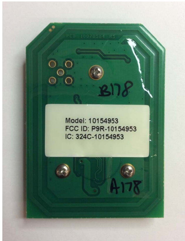
Figure 2 - FCC / IC Label Placement on RFID Module
