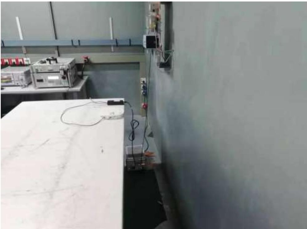
Description: Radiated Emission Test Setup for Below 1GHz(AP410C)
