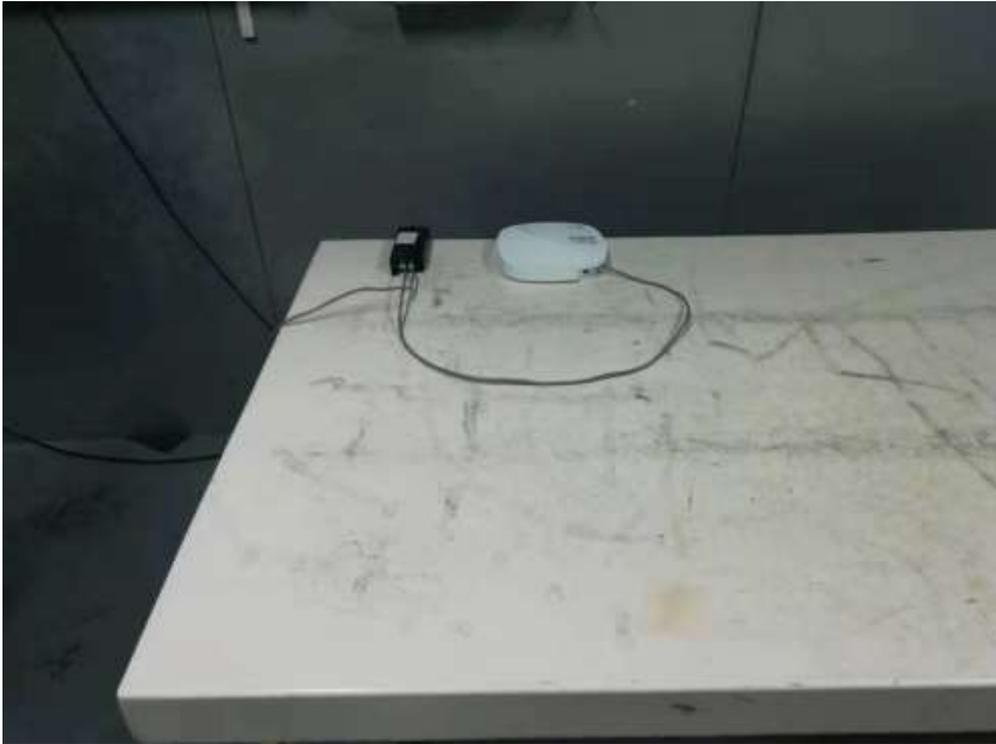
Description: Conducted emission Test Setup(AP410C)
