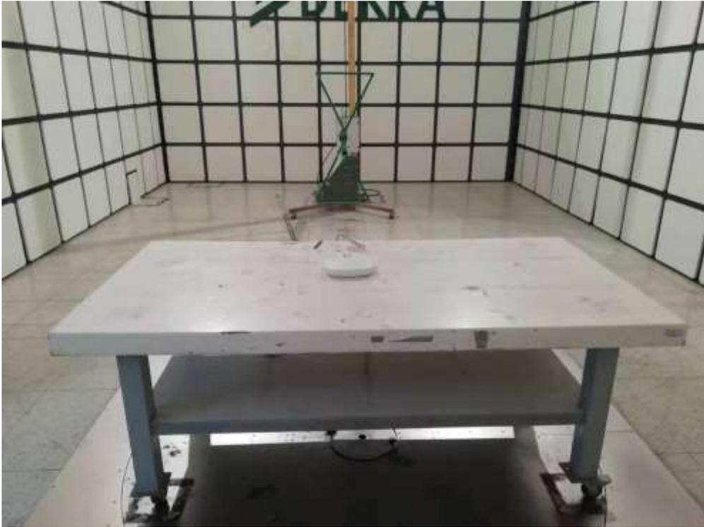
Description: Radiated Emission Test Setup for 1~18GHz(AP410C)
