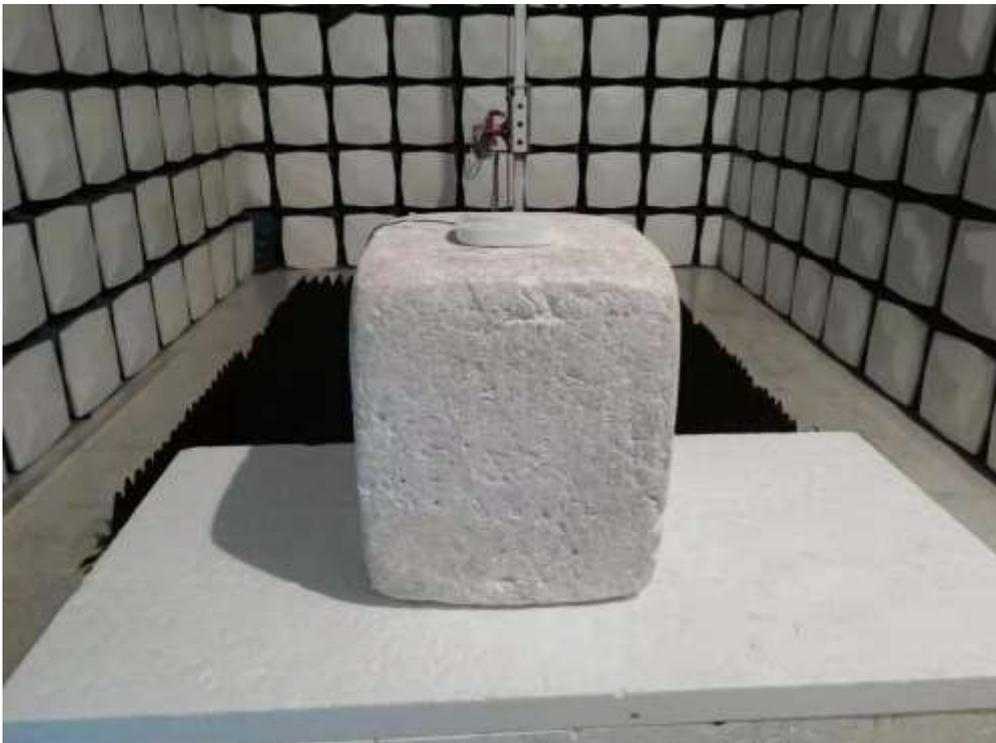
Description: Radiated Emission Test Setup for Above 18GHz(AP410C)
