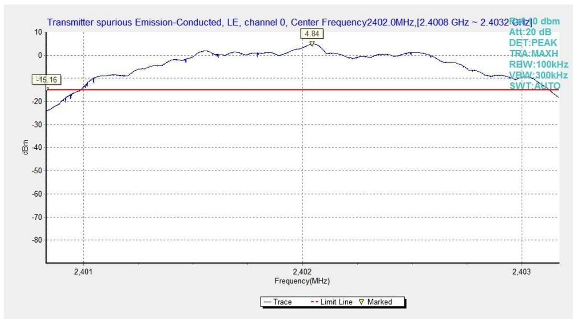
**Fig.5.** Transmitter Spurious Emission - Conducted: GFSK, 2402MHz
