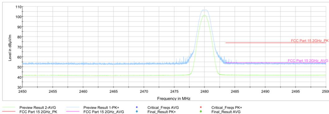
Fig.4. Frequency Band Edges: GFSK, 2480 MHz, Hopping Off, 2.45 GHz - 2.50GHz
