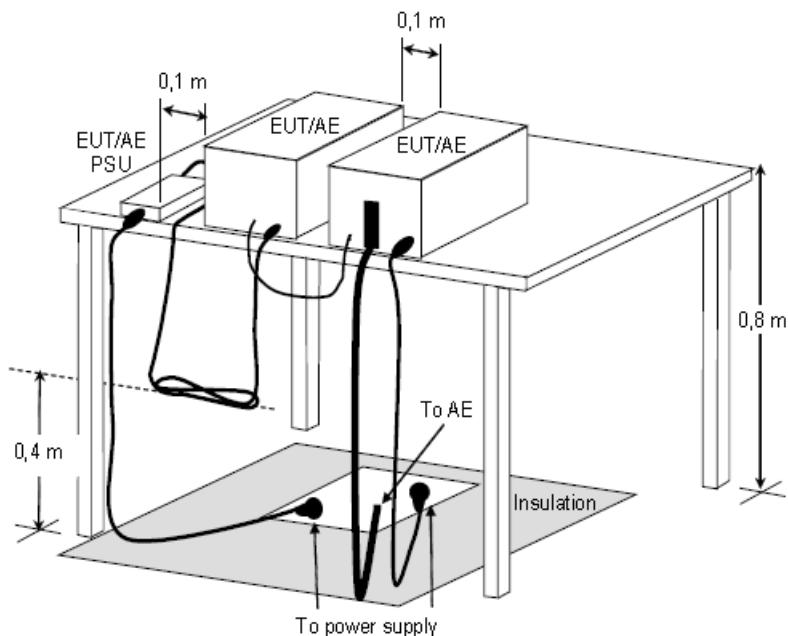
Figure D.8 – Example measurement arrangement for table-top EUT
