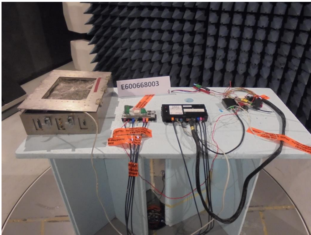
Test setup 30MHz <f <1GHz: close view
