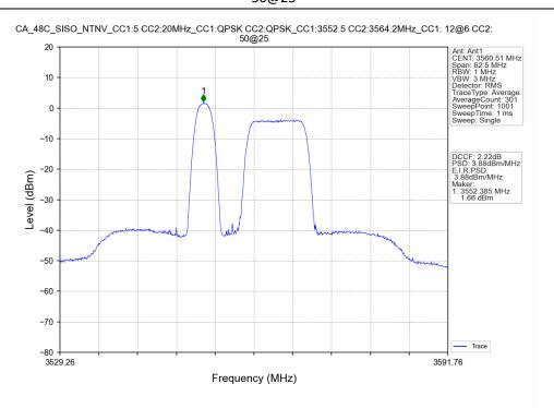
CA\_48C\_SISO\_NTNV\_CC1:5 CC2:20MHz\_CC1:QPSK CC2:QPSK\_CC1:3552.5 CC2:3564.2MHz\_CC1: 12@13 CC2: 50@50
