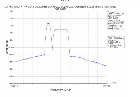
CA\_48C\_SISO\_NTNV\_CC1:5 CC2:20MHz\_CC1:16QAM CC2:16QAM\_CC1:3552.5 CC2:3564.2MHz\_CC1: 12@6 CC2: 50@25
