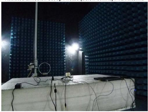
Radiated Emission Set up Photos (Below 1GHz)
