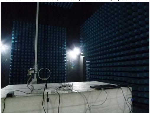
Radiated Emission Set up Photos (Below 1GHz)
