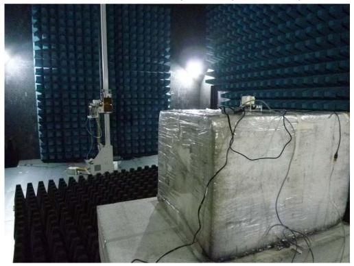
Radiated Emission Set up Photos (Front View)
