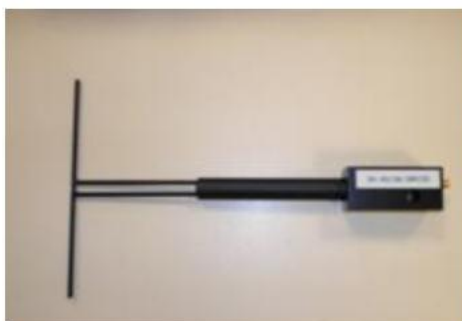
Figure 1 – Satimo COMOSAR Validation Dipole
