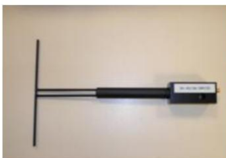
Figure 1 – Satimo COMOSAR Validation Dipole
