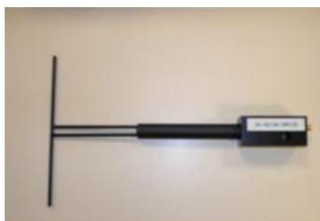
Figure 1 – Satimo COMOSAR Validation Dipole
