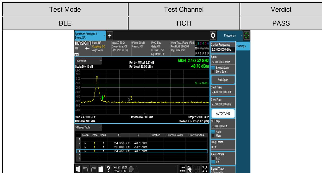
**PART 3: CONDUCTED SPURIOUS EMISSION****TEST RESULTS TABLE**
