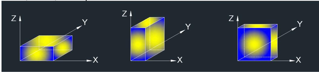
Note: For all radiated test, EUT in each of two orthogonal axis emissions had been tested, but only the worse case (X axis) data recorded in the report.
