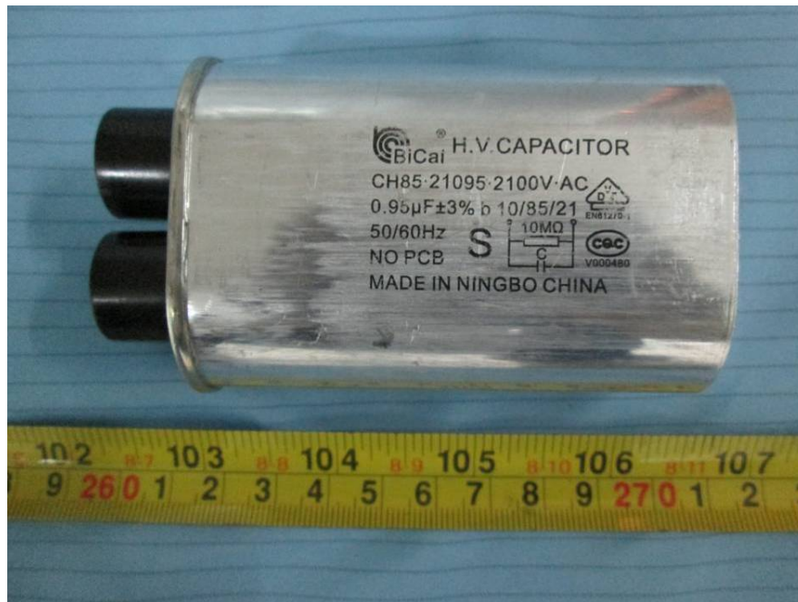
EUT – H.V. Capacitor View
