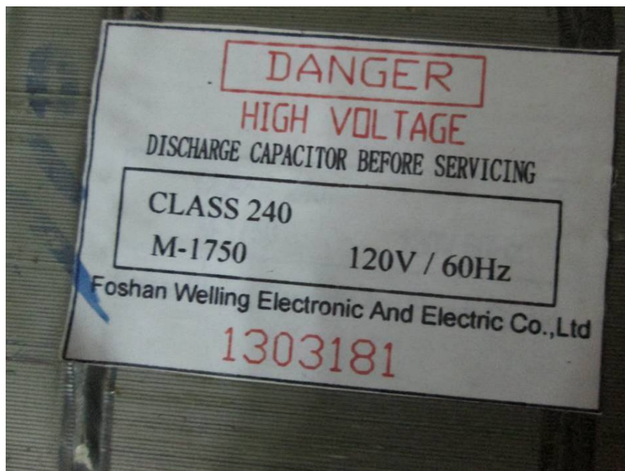
EUT – Power Transformer Label View
