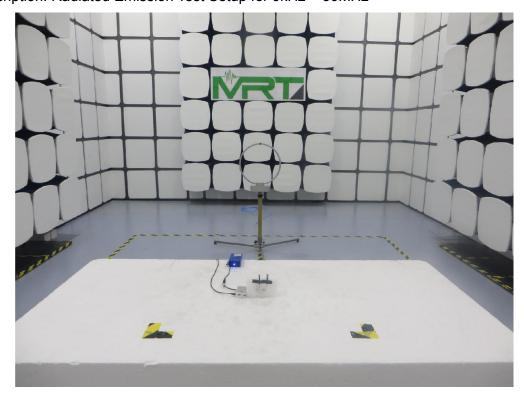
Description: Radiated Emission Test Setup for  $30 MHz \sim 1 GHz$
