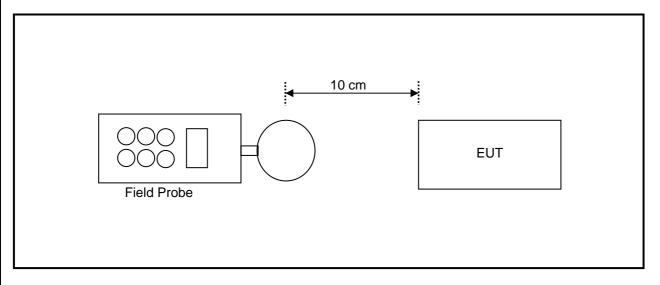
Note: Measurements should be made from all sides and the top of the primary/client pair, with the 10 cm measured from the center of the probe(s) to the edge of the device.
