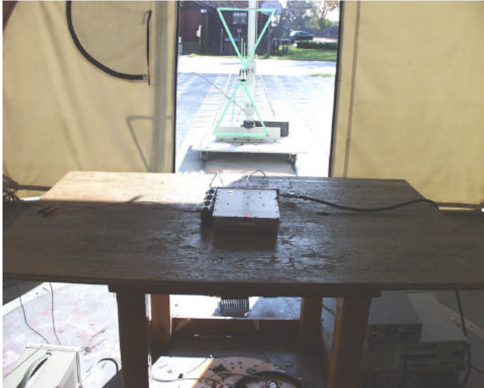
Part15 back view Radiated Emission Setup
