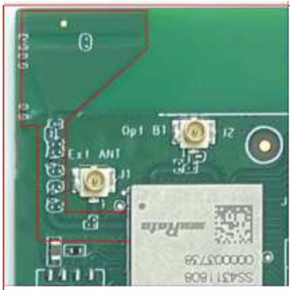
Figure 7: 50 \Omega microstrip line and Type 2FR_Antenna
