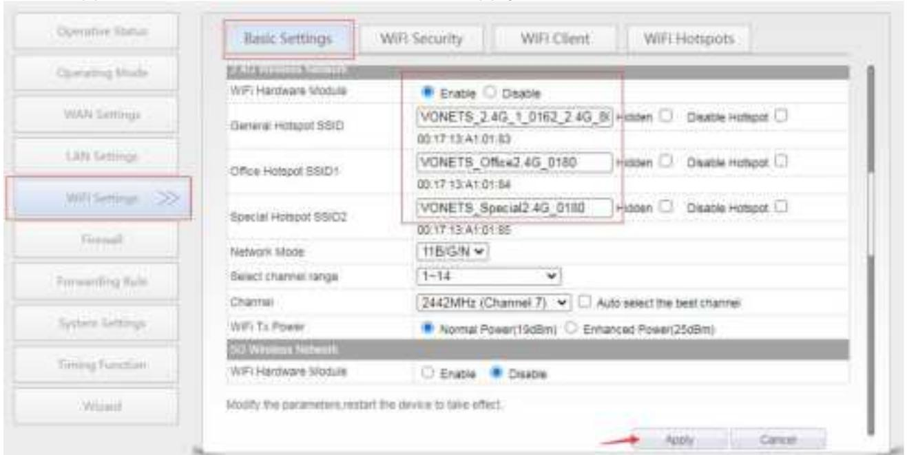
2. Change WiFi password: select "WiFi Security" in "WiFi Settings", enter a new WiFi password in the text box after the key, you can set different passwords for different hotspot names, and then click the "Apply" button;
