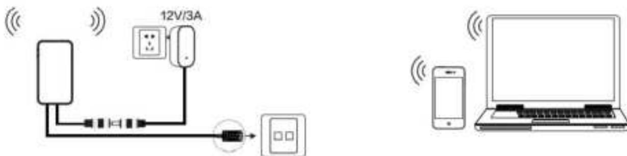
**1.2 Router Mode**(In the actual application environment, if the POE output port (PSE) is connected to a non-POE network port (PD is an access network port), please use it with caution, and ensure that the access network port is isolated from the power supply ground, otherwise it may cause the access device. damage!)
