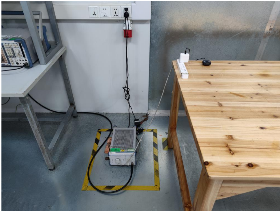
FCC ID: 2AQI5-WS108 Photo of Power Line Conducted Emission Test
