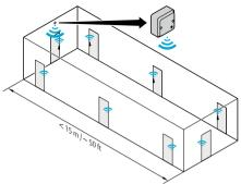
Example of placement of the Hub with 8 locks. AH40 can manage up to 16 locks.
