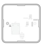
The "LINK" LED on the communication Hub indicates both status of the Ethernet Link level and if communication is ongoing. Note: LED on the Ethernet connector is not used.
