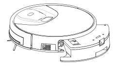
Press the release button to take out the water tank.
