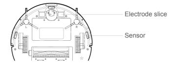
Use the cleaning tools or a dry soft cloth to periodically clean the electrode slice of robot chassis and the sensor window.
