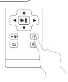
You can set the current local time on your robot by pressing the Clock Setting button on the remote controller, then press Confirm button.
