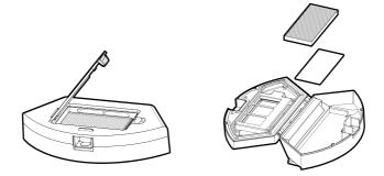
Open the high-efficient filter cover, and remove the high-efficient filter and filter sponge. It is not recommended to wash the high-efficient filter with water. Please pat off the debris carefully.
