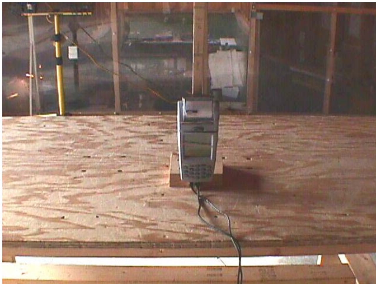
Radiated Emissions at 3 Meters Distance Orthogonal Position # 3
