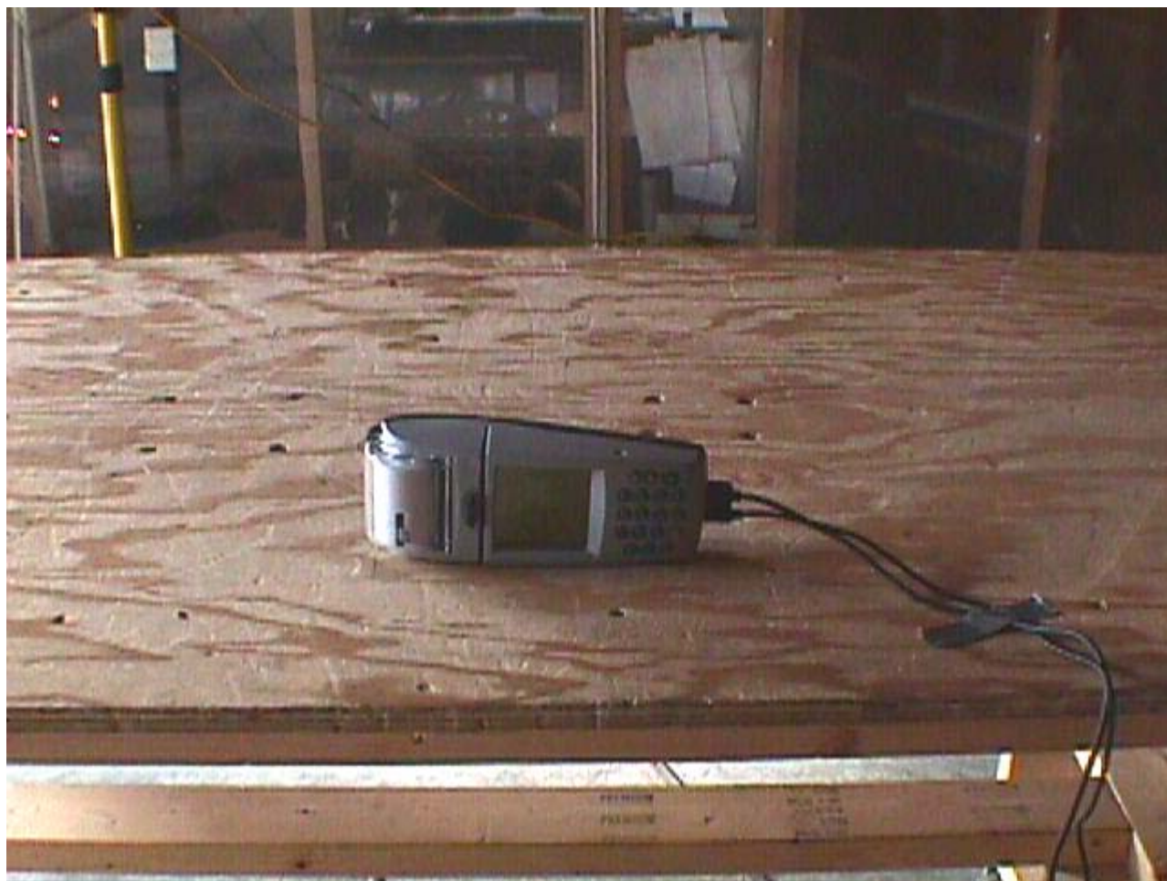
Radiated Emissions at 3 Meters Distance Orthogonal Position # 2
