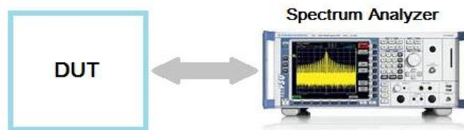
Radiated emissions test setup 9 kHz – 30 MHz
