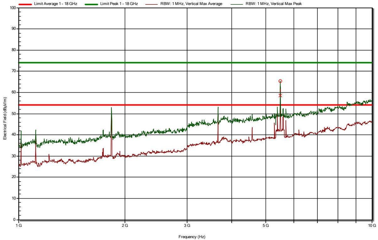
**Note:** The harmonics seen in the plots above are falls inside of restricted bands of operation defined in Part 15.205 of the FCC regulation. Thus as described in FCC Part 15.247 sub-section (d) the actual applicable limit shall be 20 dB lower of the actual transmitter peak value which is 94.39 dBµV/m for this case.
