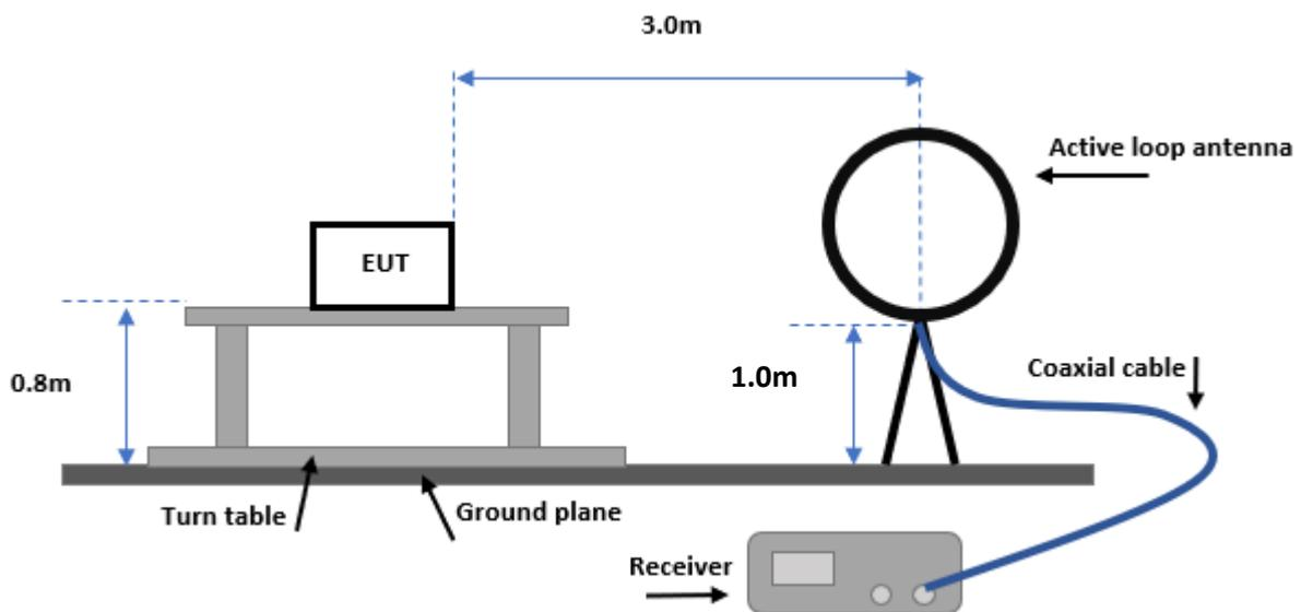
**Radiated emissions test setup 30 MHz - 1 GHz**
