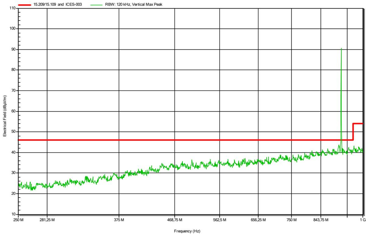
Note: The peaks in the 902 - 928 MHz range seen in the plots above are the transmission frequencies and therefore not subject to the spurious limit.
