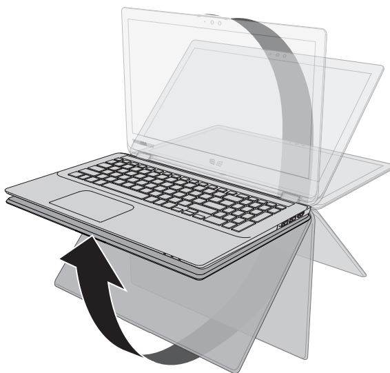
Figure 2-1 Opening the display panel to any angle
