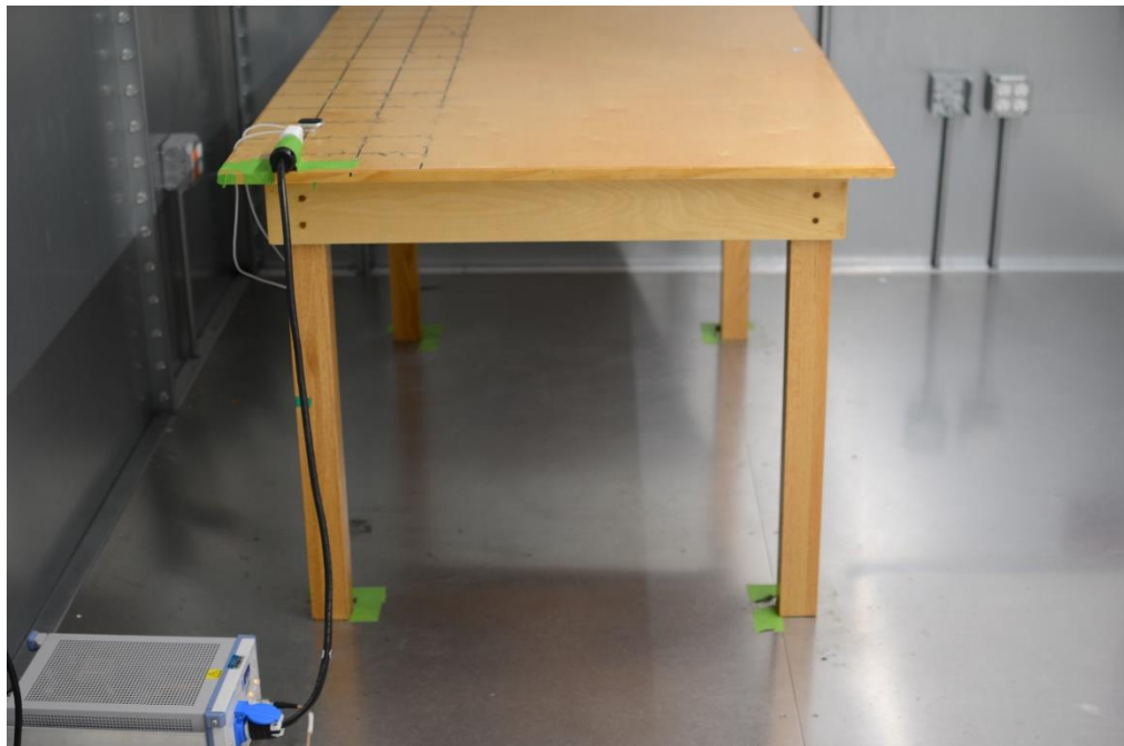
Figure 2: AC Line Conducted Emissions (Side View)
