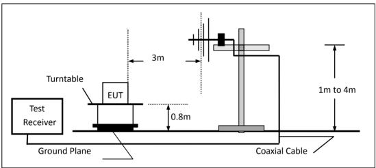
(c) For radiated emissions above 1000MHz
