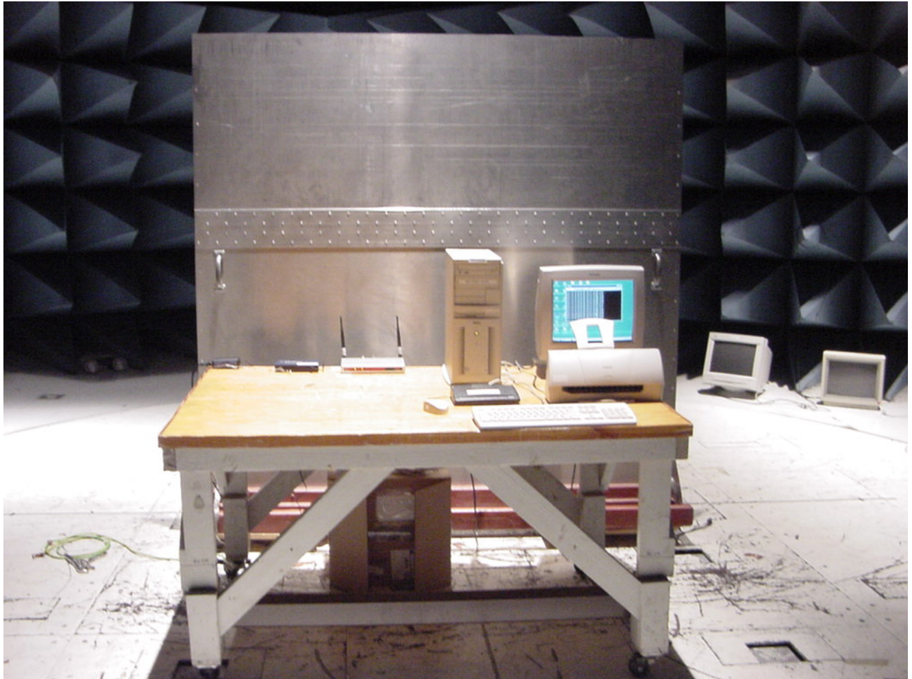
Photograph 1. Conducted Emissions Test Setup
