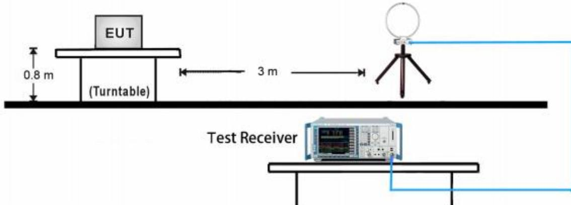
30MHz ~ 1GHz Test Setup:
