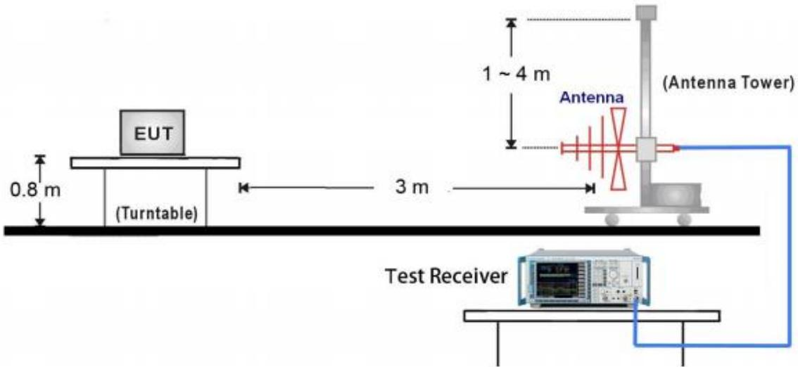
1GHz ~ 18GHz Test Setup:
